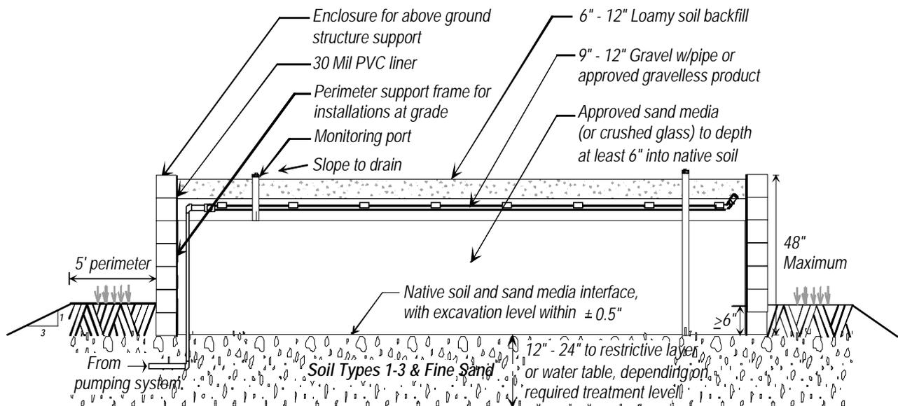
**Figure 6 – Example of Bottomless Sand Filter Enclosure
