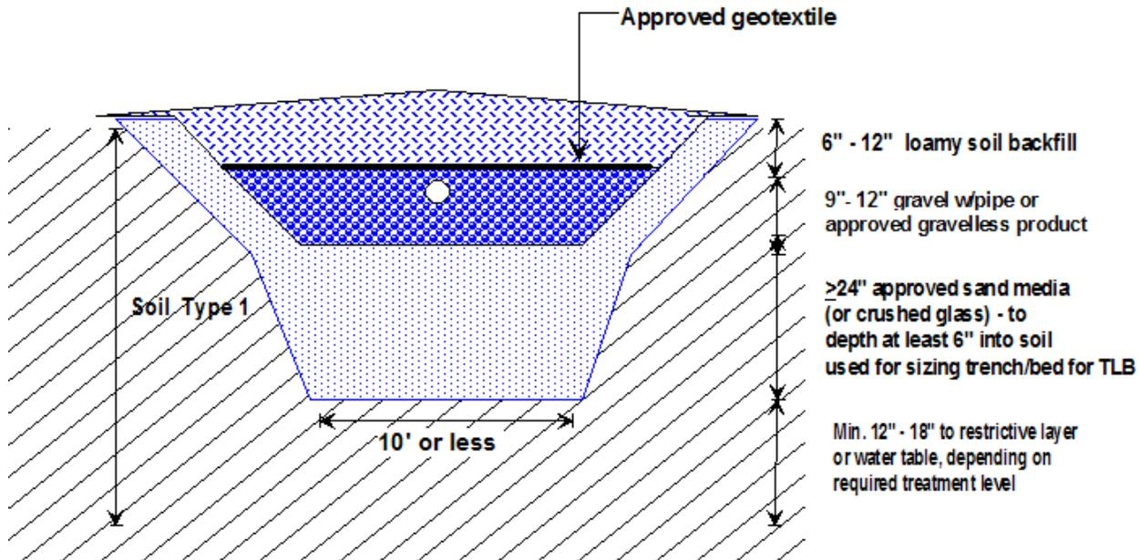
**Figure 2.4 - Type 1 Soil Extending up into Trench/Bed Zone (Option 3)
