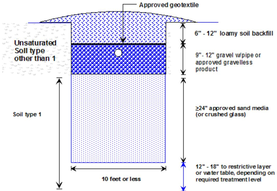
**Figure 2.2 - Type 1 Soil Extending up into Trench/Bed Zone (Option 1)**
