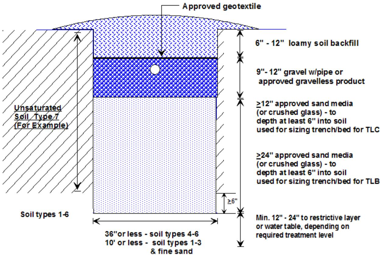
**Figure 4 – Bottomless Sand Filter**
